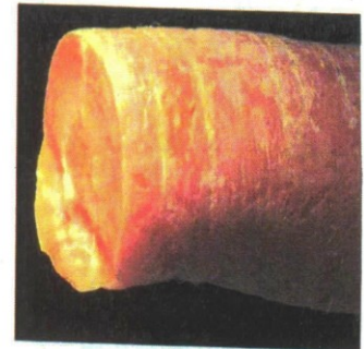
Fig. 1 – Carrot fractured in three-point bend test. The crack is perpendicular to the length of the specimen, except at the last portion to separate. This "hinge" may have parallels to shear lips in metal specimens.
